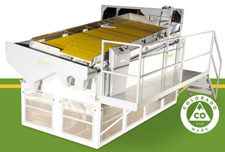
This maximum capacity gravity separator raises the bar with its advanced touchscreen accessibility and is ready for the modern world of particle separation. The Oliver Maxi-Cap Platinum series brings the safety, simplicity and efficiency of integrated control to one of the most reliable gravity separators ever made. The advanced touchscreen provides simplified operation, reduce yield losses due to human error, and pinpoint airflow to bring to you the highest quality end product possible.
