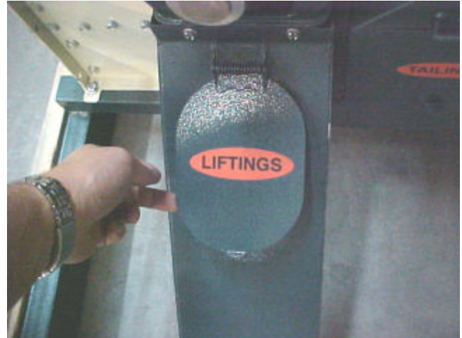
Large Inspection Ports
