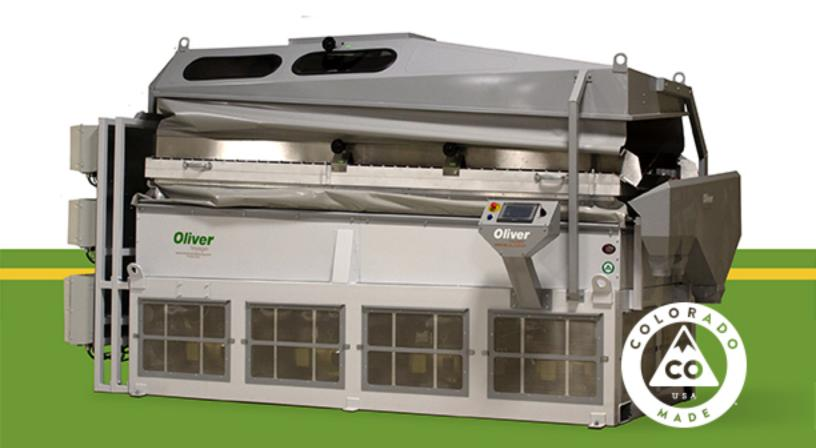
The Oliver Voyager continues to set the industry bar for precision density separation. With advanced touchscreen accessibility, the Voyager series is ready for the modern world of particle separation. Adjustable controls make adapting to product throughput easier and more convenient. Oliver's signature rectangular deck design, a company standard, maximizes the quality of your product separation, and the multifaceted fan system allows for precise airflow control.
